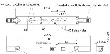
M5 Holes for Possible Side Fixing to Extrusion
