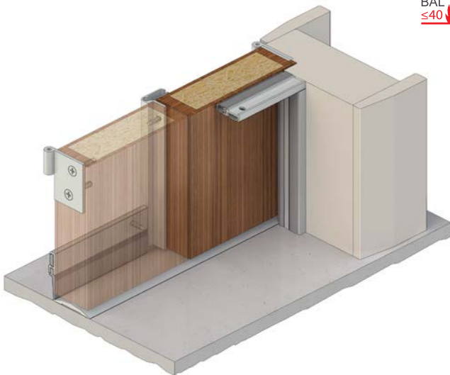
Double Outward Opening Doors
